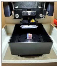
Specimen tray fixed on buffer tray
